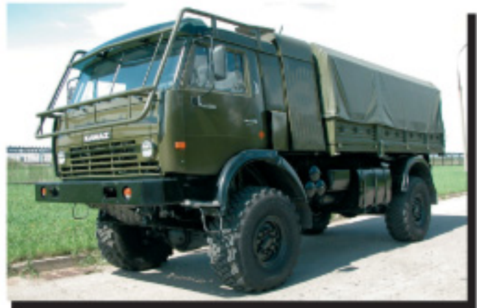
KAMAZ-4911 (4x4) 4 ton Fast Command Vehicle, Engine 730 HP
