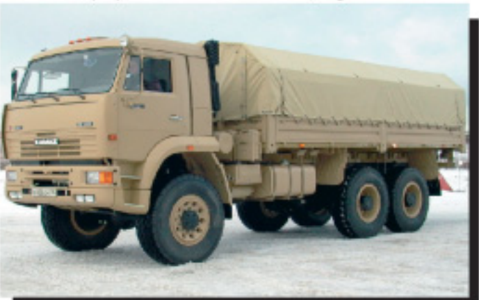
KAMAZ-65224 (6x6) 14 ton Heavy Gun Tower, Engine 360 HP
