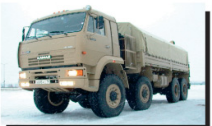
KAMAZ-6560 (8x8) 19 Ton Heavy Gun Tower, Engine 400 HP
